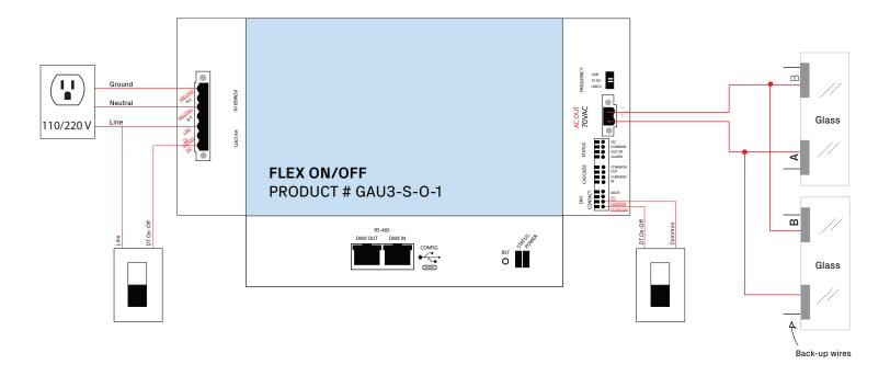
**WARNING:** Never connect high voltage (110/220 VAC) to the dry contact interface. Doing so will permanently damage the controller.
