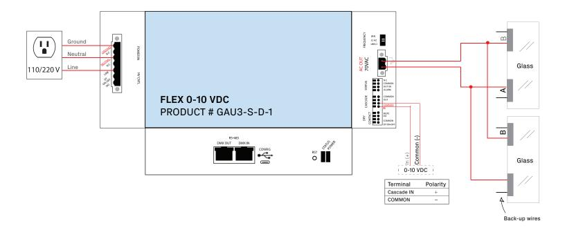
**WARNING:** Never connect voltage higher than +10 VDC to the cascade interface. Doing so will permanently damage the controller.
