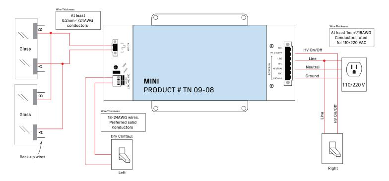
**WARNING:** Never connect high voltage (110/220 VAC) to the dry contact interface. Doing so will permanently damage the controller.
