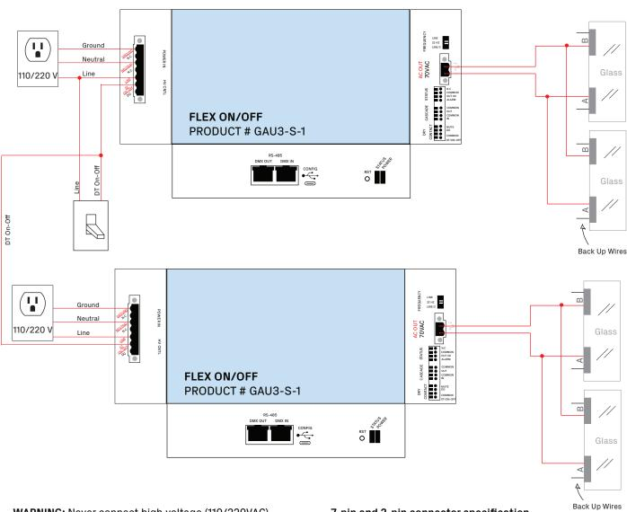
**WARNING:** Never connect high voltage (110/220VAC) to the dry contact interface. Doing so will permanently damage the controller.
